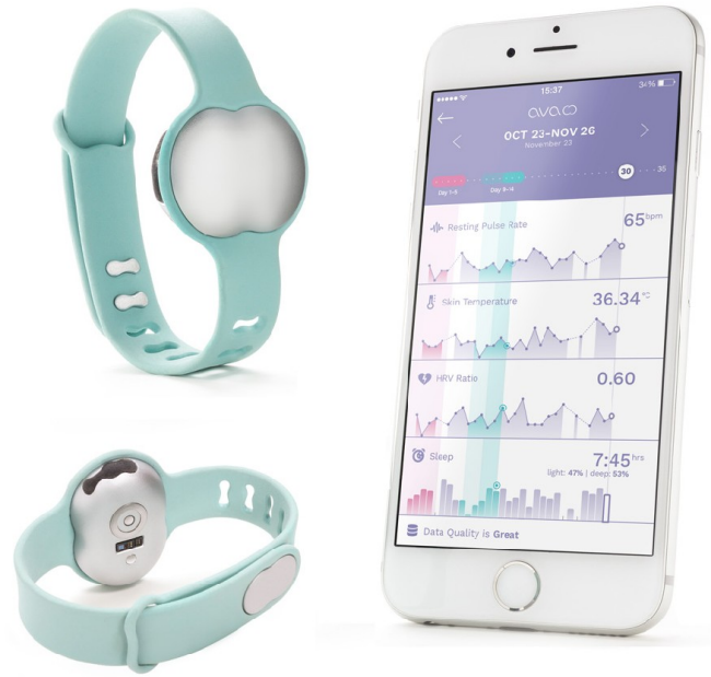
Fig. 1. Ava bracelet with a multi-wavelength PPG sensor to record beat-to-beat intervals.
